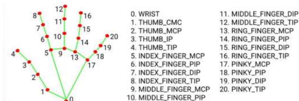
Figure 2 Localization of key points using media pipe
